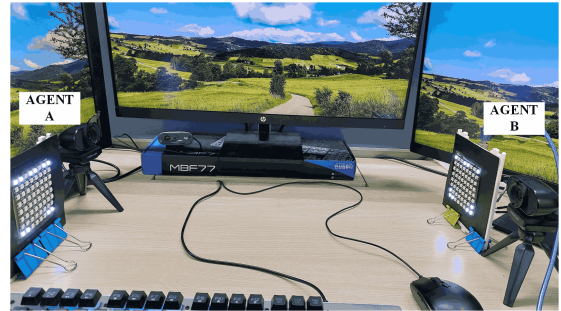
Fig. 4. Experiment setup with initial distance between agents is 0.5 meter.
