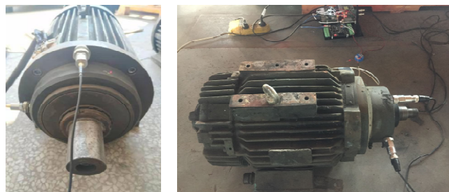
Fig. 3. Grinding Motor Data Collection
